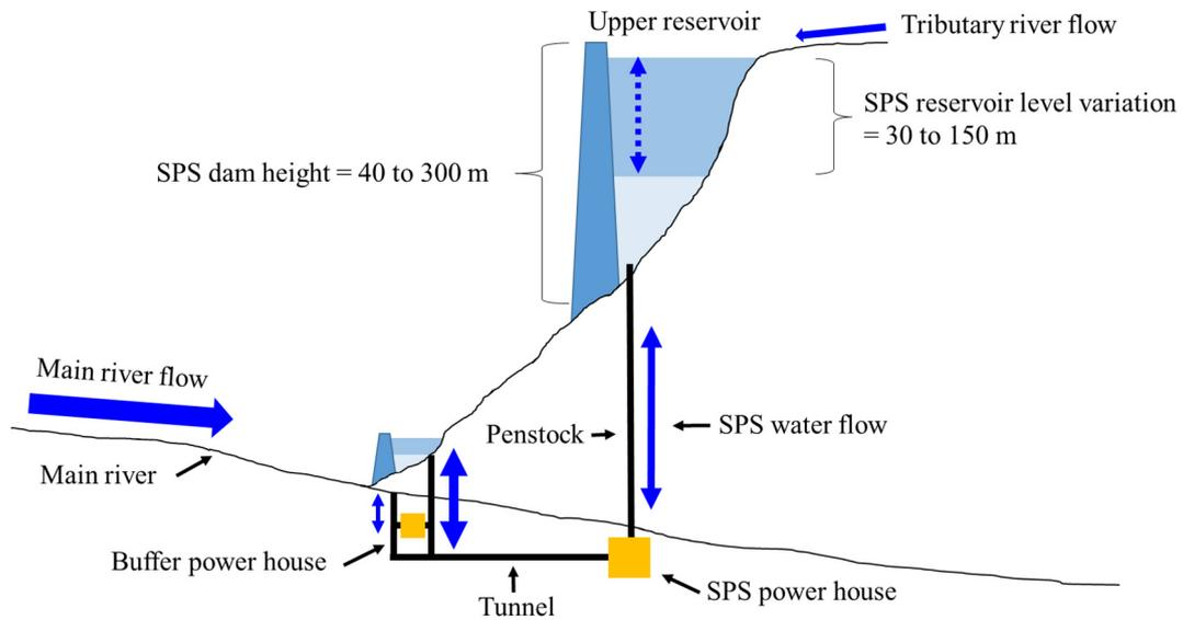
Fig. 7. Schematic presentation of the Run-of-the-River Seasonal Pumped-Storage.
