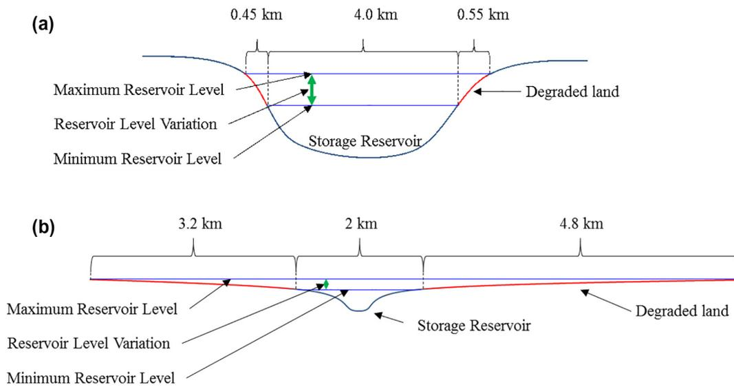
Fig. 2. Comparison of reservoirs with a (a) steep valley, and (b) shallow topography.
