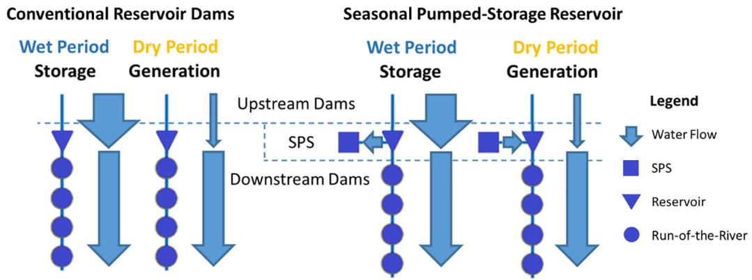
Fig. 5. Diagrams presenting (a) reservoir hydropower dams and (b) seasonal pumped-storage.
