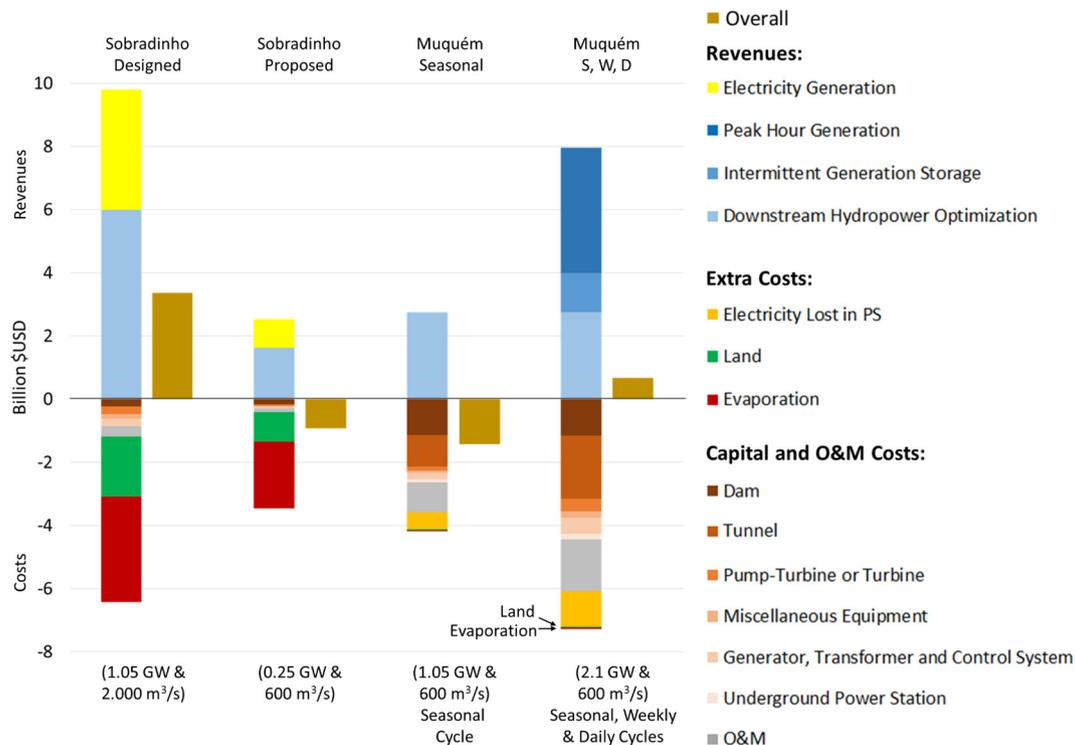
**Fig. 10.** Overall cost estimates for Sobradinho CRD with 2000 m<sup>3</sup>/s (1.05 GW) and 600 m<sup>3</sup>/s (0.25 GW) and Muquém SPS plant with 1.05 GW and 2.10 GW generation capacities over 40 years.
