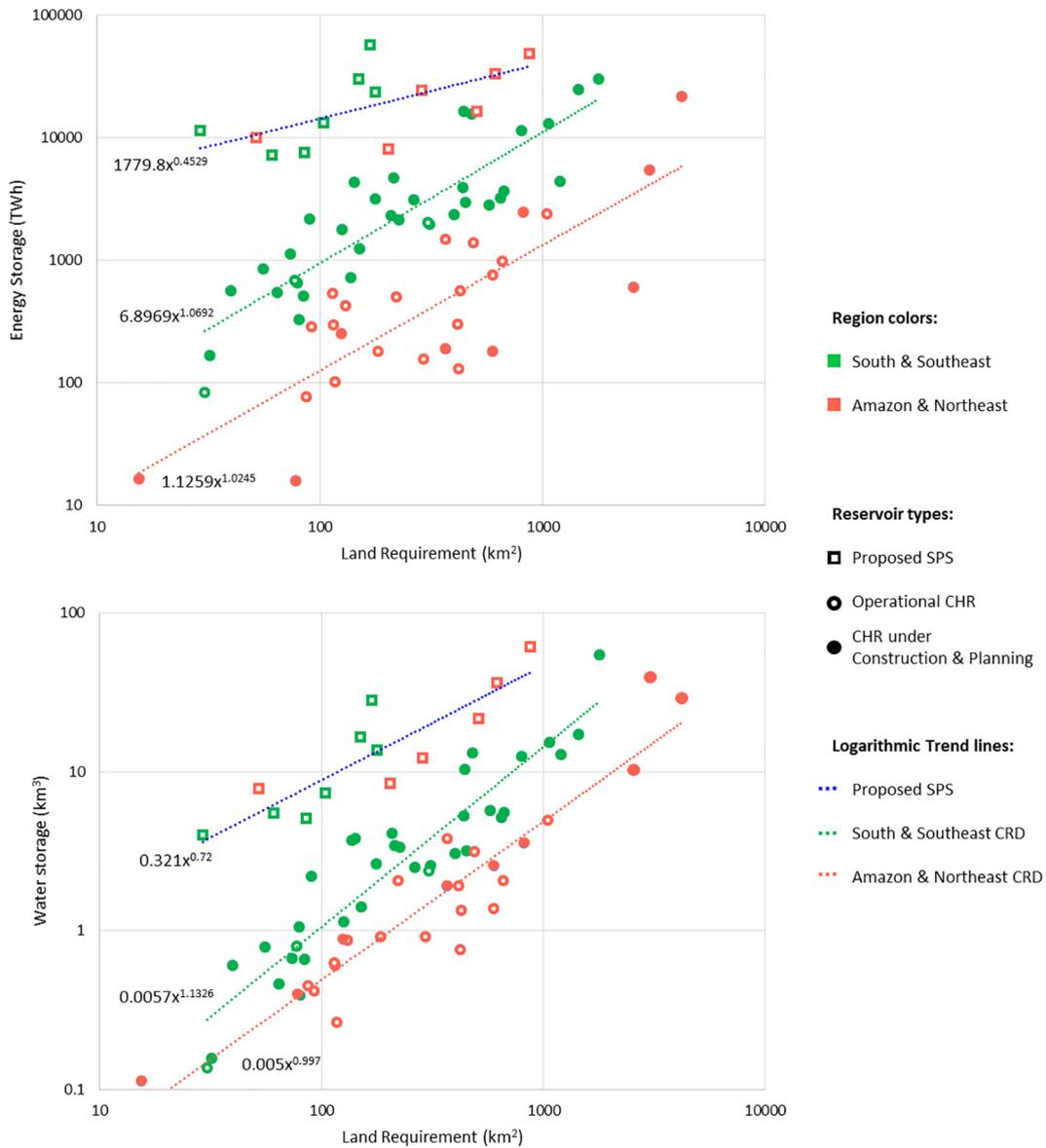
Fig. 12. Comparison between energy storage (upper graph) and water storage (lower graph) and land requirement in CRD and SPS in Brazil.
