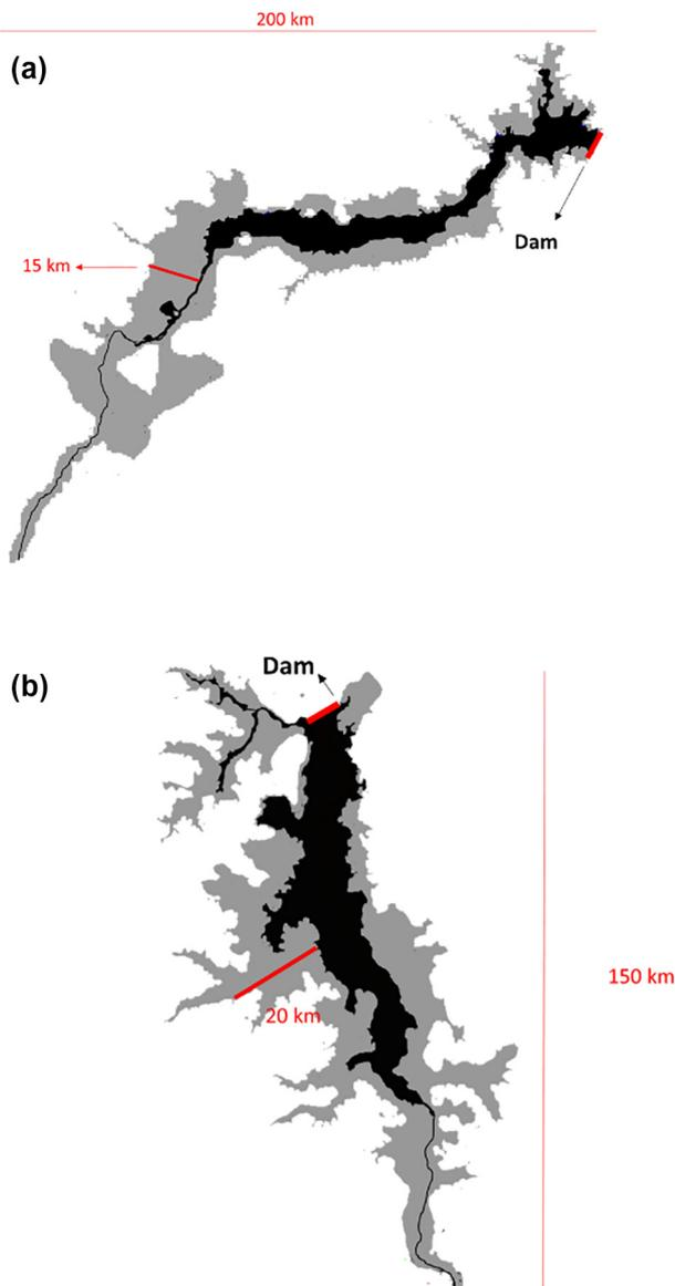
**Fig. 3.** Flooded area variation of (a) Sobradinho and (b) Tucuruí reservoirs in Brazil (see Fig. 11) when full (gray) and when reaches dead storage (black) [49,50].
