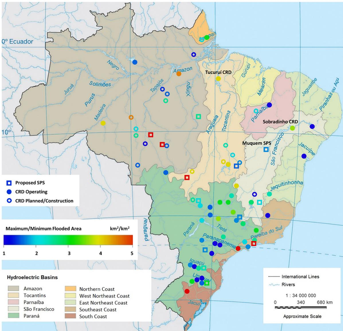
Fig. 14. Ratio between reservoir maximum and minimum flooded area ratio for CRD dams and SPS, representing the difference between the full and seasonal minimum capacity.
