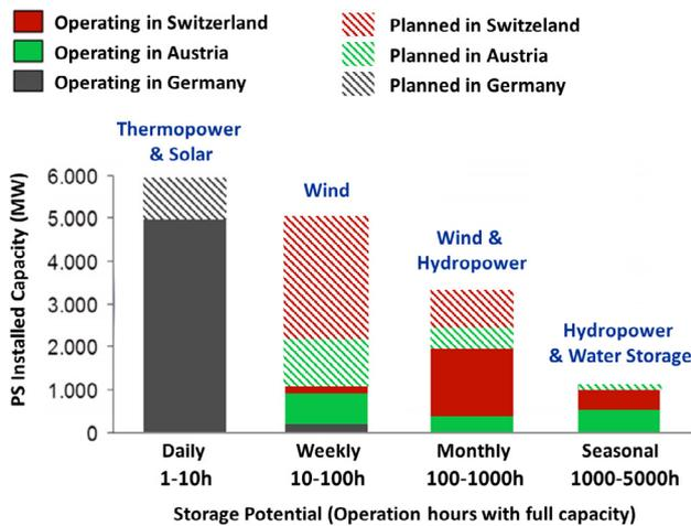
**Fig. 4.** Operating and planned pumped-storage potential in Germany, Austria and Switzerland, including the main purposes of the storage cycles (). adapted from [66]
