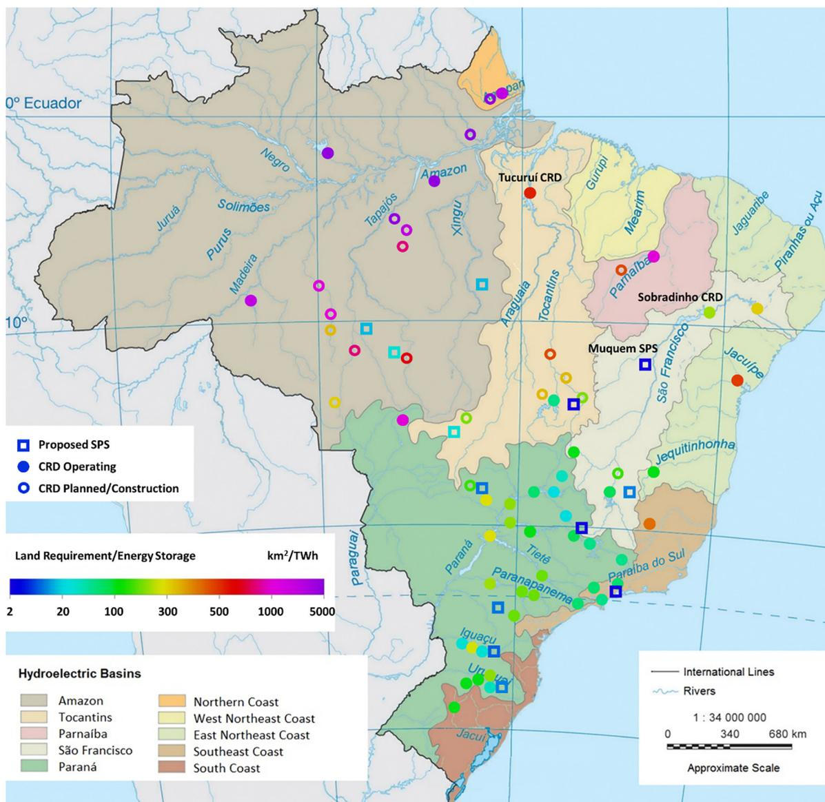
Fig. 11. CRD and SPS reservoir land requirement for energy storage.
